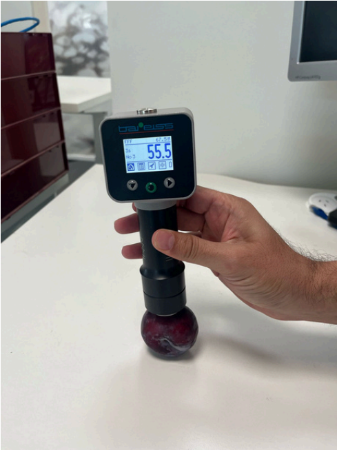
Figure 2. Ultra-Precision Digital Durometer HPE-III-FFF determines non-destructive fruit flesh firmness
