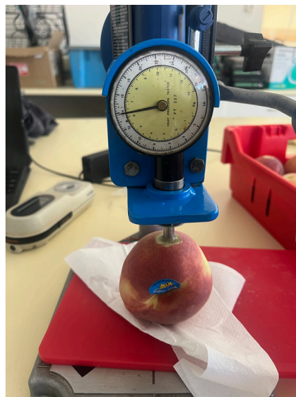
Figure 1. (A): Hand-held penetrometer mounted on a Dremel workstation.
