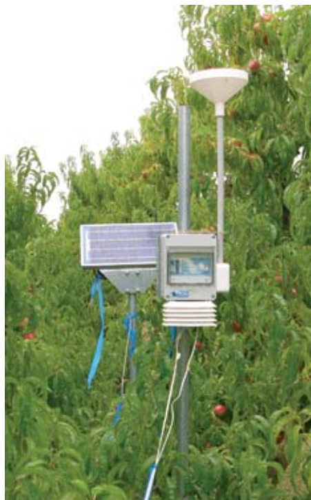
Automated weather stations enable site-specific disease risk assessment
