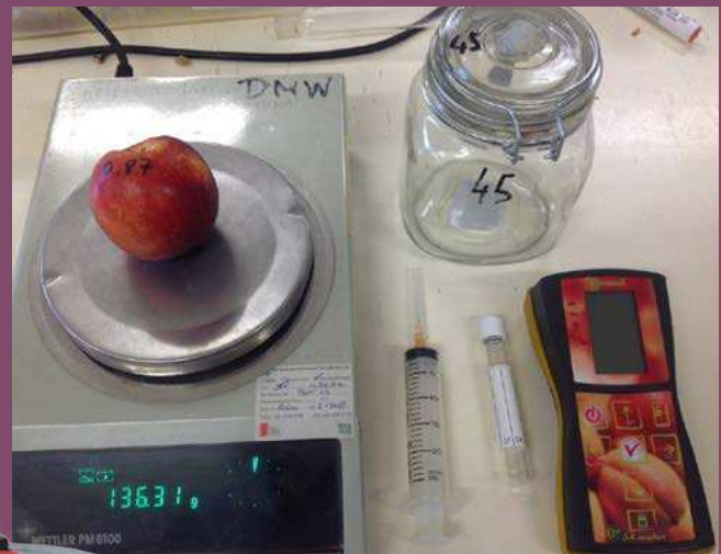
ABOVE: Equipment needed to perform the procedure of sampling fruit ethylene. A example of a glass chamber of approximately 1L volume. LEFT: Example of plastic chamber of approximately 1L volume.
