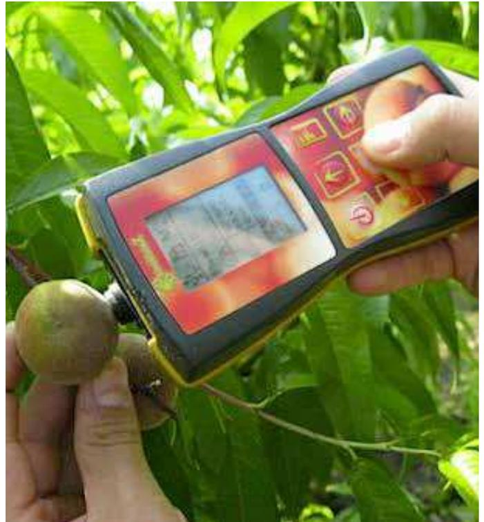
The DA meter can be used to track how fruit are developing and maturing on the tree. Photo: DEDJTR
