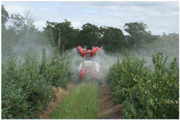
Quantum mist spray unit in a blueberry crop minimises spray drift and fans direct drops onto the target crop saving refill time and spray volume.
