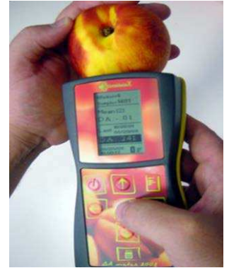
Figure 3. Non-destructive DA meter for measuring peach and nectarine fruit maturity using index of absorbance ( I_{AD} ).
