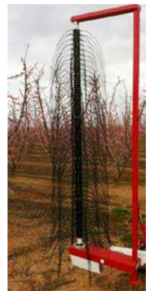
Figure 2. Darwin 300 mechanical string thinner mounted on a tractor used for
