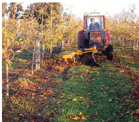
Figure 146. The 'Sadie' sweeper in action moving leaf and pruning residue to the centre of the row for mulching Photo: Crendon Machinery.
