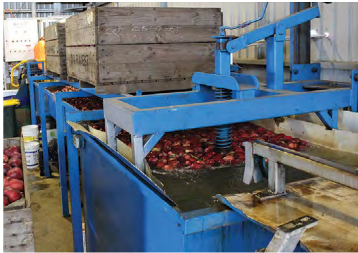
Figure 179. Dipping or drenching fruit in a fungicide solution as it comes into the packing shed.
