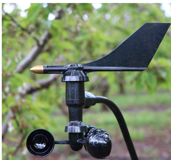
Figure 4. Davis Vantage Pro Anemometer installed at the Nashdale trial site.
