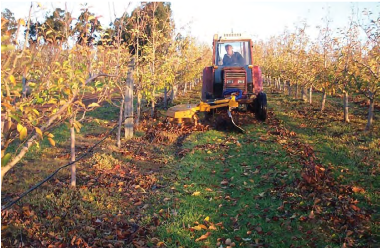
Figure 18. Tractor-mounted orchard sweepers help move fallen leaves into the inter-row, where they can be mulched into smaller pieces to accelerate their breakdown.
