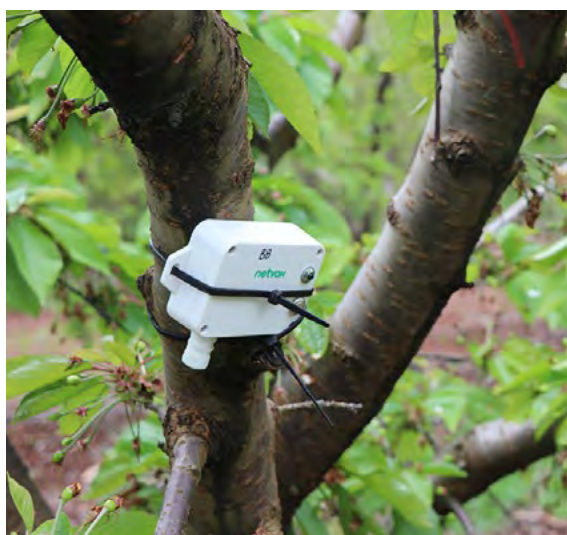
Figure 5. Netvox R718A temperature and humidity sensor installed at the Nashdale trial site.
