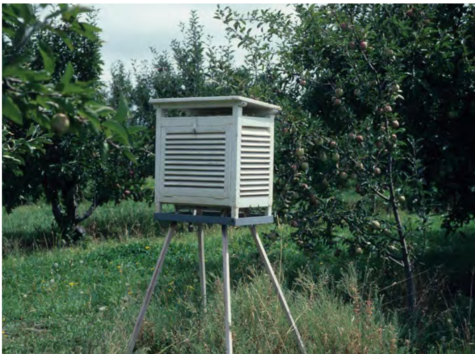
Figure 138. A Stevenson screen is the recommended housing for temperature recording in the orchard.
