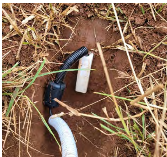
Figure 6. Meter Teros-12 soil moisture probe installed at the Nashdale trial site.
