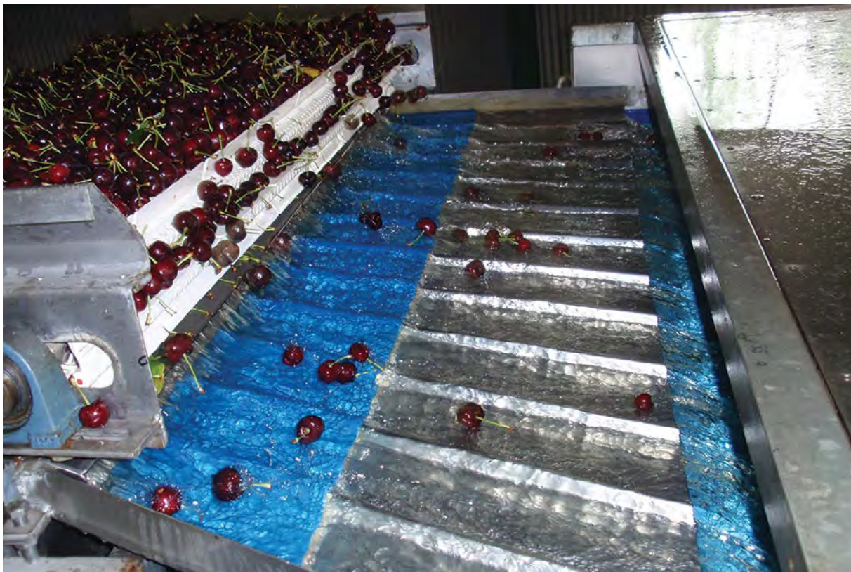
Figure 180. Sanitising water transport systems is essential to prevent the build-up and spread of fungal and bacterial infections.
