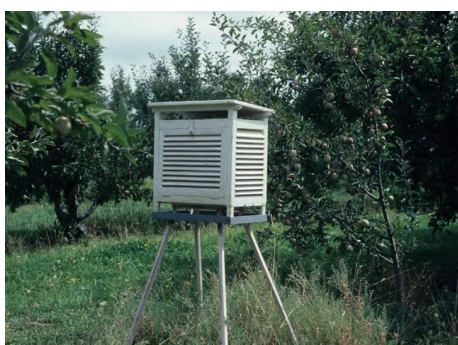
Figure 1: A Stevenson screen -recommended housing for temperature recording in the orchard.
